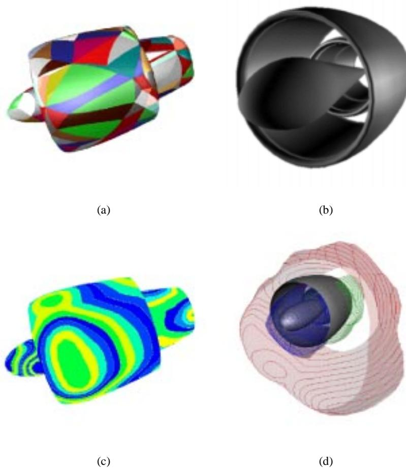
Figure 6: A jet engine. (a)  $C^0$  reconstructed domain. Patches are visible in different colors. (b) Reconstructed domain (after  $C^1$  smoothing). (c) Iso-pressure contours and regions of a surface-on-surface pressure function displayed on the surface of the jet engine. (d) The reconstructed engine surface and visualization of the pressure surface function surrounding the jet engine using the normal projection method.
