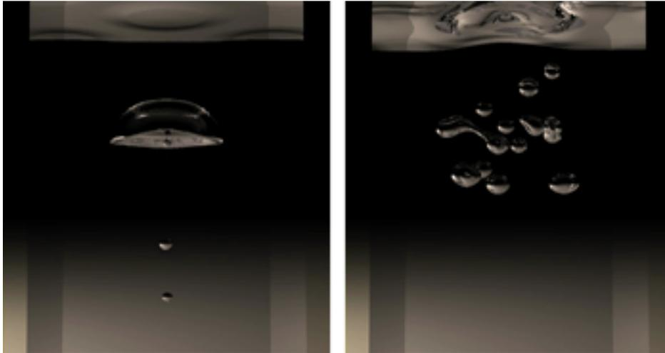
**Fig. 1** (left) An air bubble rising in calm water; (right) air bubbles spiraling upwards
