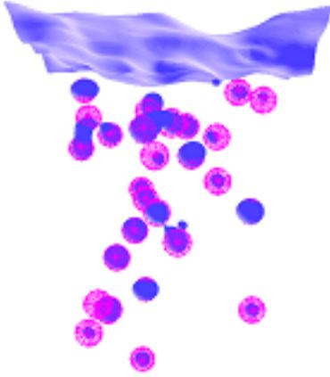
**Fig. 3** Bubble particles are seeded in every air bubble; the red spheres in this three dimensional example are bubble particles
