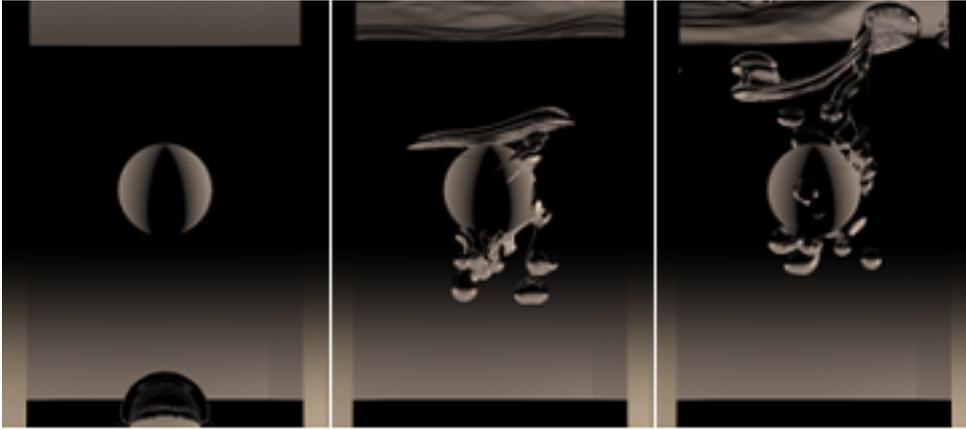
**Fig. 5** Rising air bubbles with bubble particles interacting with a rigid sphere
