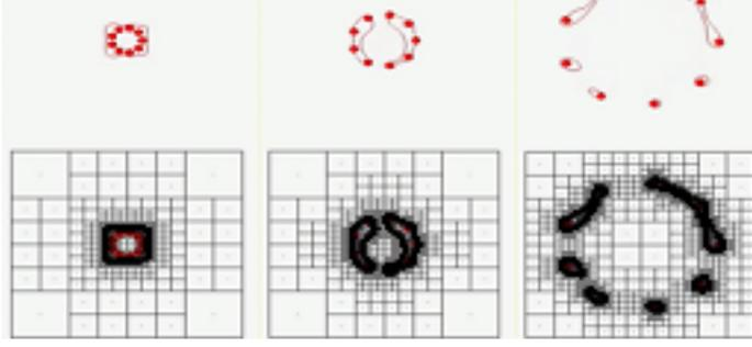
**Fig. 2** Level set changes in evolving bubble particles (in two dimensions).
